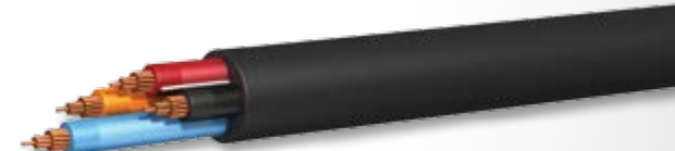
Tray Cable - Power and Control Cable - with or without Ground - THHN/XHHW-2/RW90 Inners Copper conductors available in 14 AWG-2 through 750 KCMIL-4, Aluminum conductors available in 6 AWG and larger
