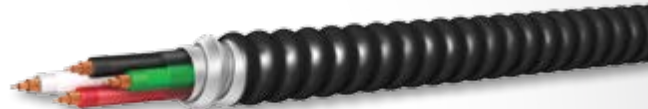
MC - PVC Jacket (AIA) THHN/XHHW-2/RW90 Inners Available in 14 AWG-2 conductor through 750 KCMIL-4 conductor with or without a PVC jacket
