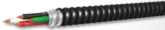
MC - PVC Jacket (AIA) THHN/XHHW-2/RW90 Inners Available in 14 AWG-2 conductor through 750 KCMIL-4 conductor with or without a PVC jacket
