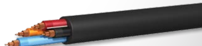
Tray Cable - Power and Control Cable - with or without Ground - THHN/XHHW-2/RW90 Inners Copper conductors available in 14 AWG-2 through 750 KCMIL-4, Aluminum conductors available in 6 AWG and larger
