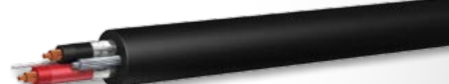
Tray Cable - Control or Instrumentation - Shielded - THHN/XHHW-2/RW90 Inners Available in 18 AWG-2 conductor through 10 AWG-12 conductor; Copper only
