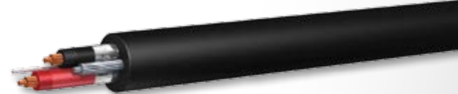
Tray Cable - Control or Instrumentation - Shielded - THHN/XHHW-2/RW90 Inners Available in 18 AWG-2 conductor through 10 AWG-12 conductor; Copper only
